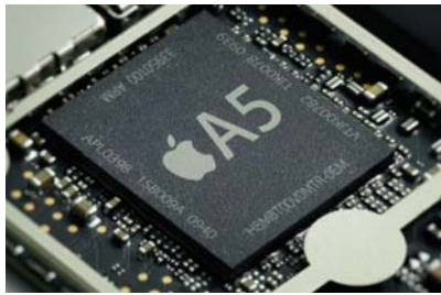
Figure 4 Apple's recently introduced dual-core 1-GHz A5 CPU (a) forms the processing nexus of the company's iPad 2 (b), although SOC specifics are currently scant.
